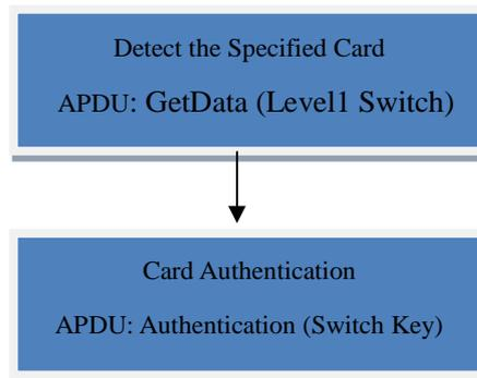
Note that to switch from the Level1 to the other Level, the detected Card Type via GetData is different. If you want to switch Level1 to Level2, then the Switch key is Switchkey2.
