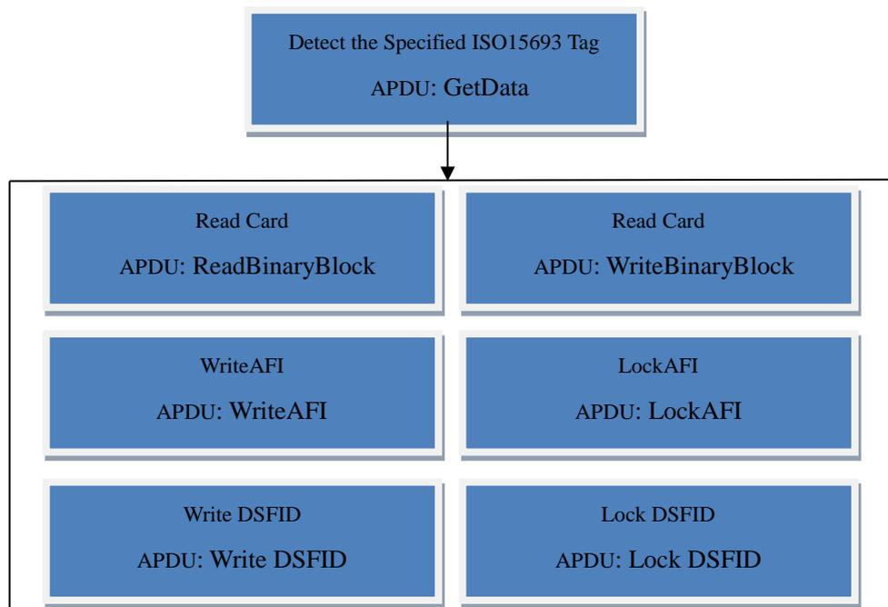
The operations for ISO15693 Tag are via "ReadBinaryBlock" and "WriteBinaryBlock" APDU commands. It's just suitable for the last detected one Tag. If you need to operate one tag which is specified the UID, please refer to the Non-Standard APDU (Custom Parts).
