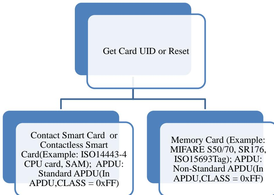
Before to operate any card, first you need send GetData APDU command to obtain the card basic information (Card serial number, reset information, etc.). GetData command contains the type of card to be switched, so once this APDU command executed, the current reading card type is also chosen.
