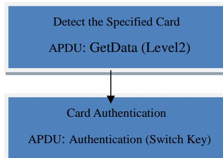
If you want to switch Level2 to Level3, then the Switch key is Switchkey3.
