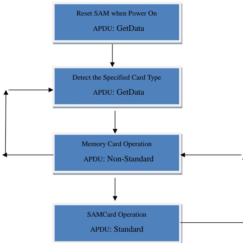
For the memory cards and single SAM operation are no need to be switched. If you need operate more than one SAM card, then before to operate this SAM card, it needs to be switched to the specified SAM card via SwitchSmartCard APDU command.
