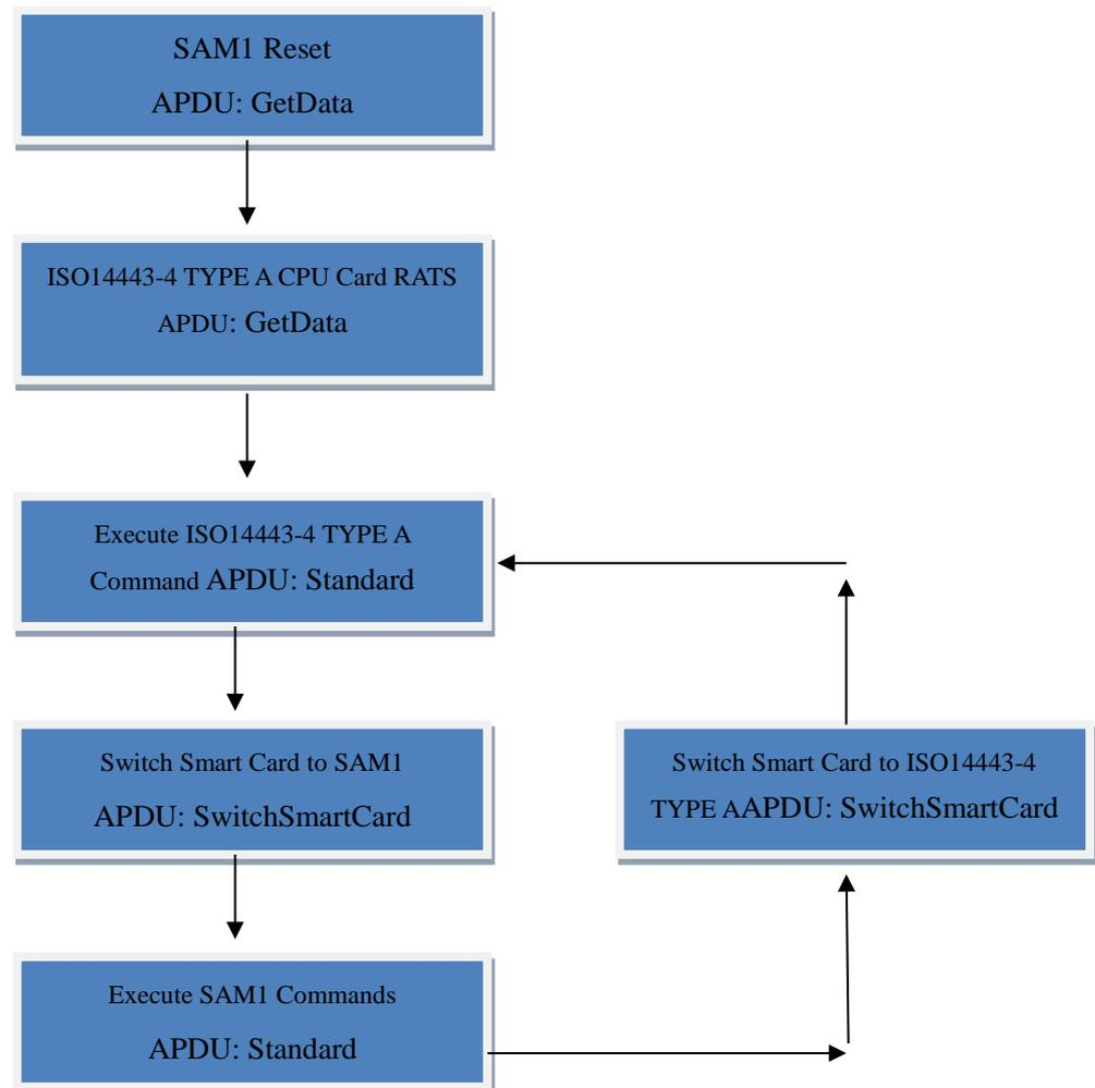
For Contact and Contactless Smart Cards, the operations are both using the standard APDU. After reset the SAM card, if you still want to operate it, and you need switch the current operated smartcard to SAM card by using the SwitchSmartCard command. To make sure the data was sent to the specified Card Type. If the Smart Card and the Memory Card do not need be switched, then after the GetData operation, now the Card type is the GetData operation Card type.
